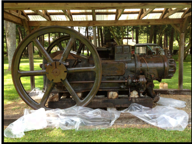
Drake Well's Reid Type DC Convertible Twin Two-Cycle engine, seen here at the time of its arrival in 2002. The engine is scheduled to undergo maintenance to make it operational.
